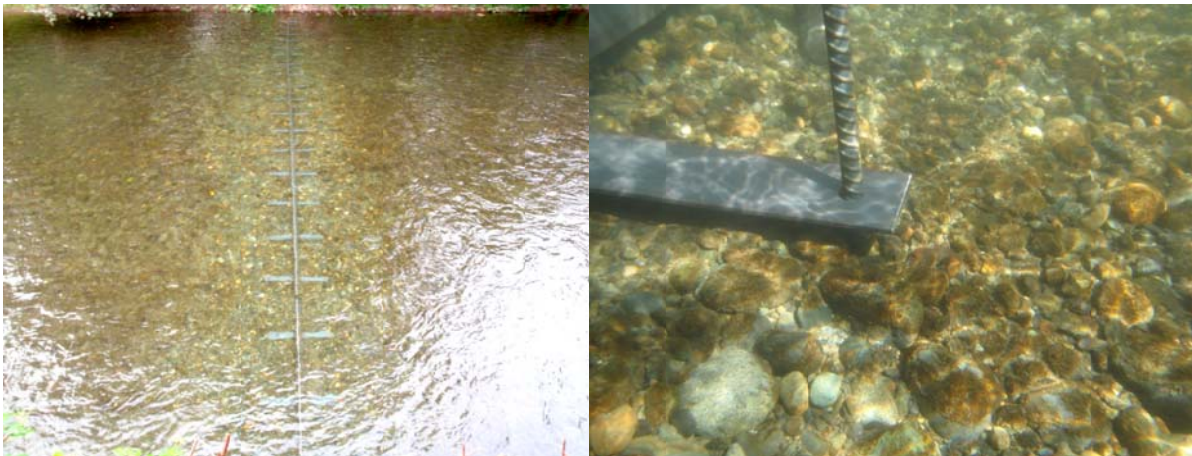
Figure 7. Installed substrate rails across river channel and substrate rail leg with inserted pin.
