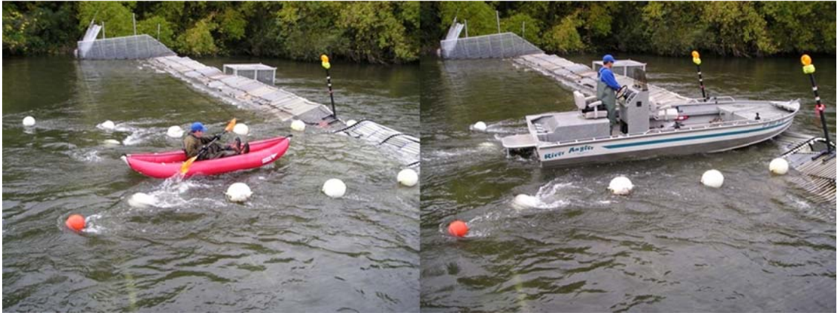
Figure 12. Inflatable kayak passing a weir (left); inboard jet boat passing a weir (right).
